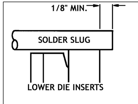
4. Depress foot switch and crimp solder.
