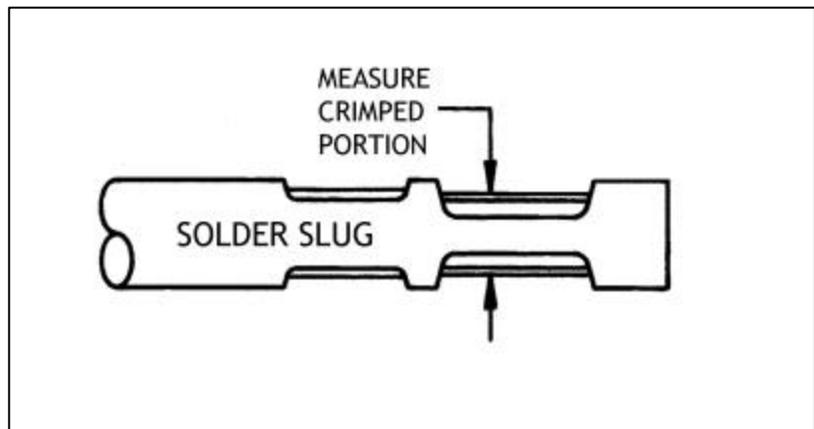
If the crimp shut height dimension is more than  $.004"$  ( $.10\text{mm}$ ) greater than the product reel label shut height dimension, then the wire crimp dial must be turned counterclockwise to the lower letter to decrease the crimp shut height.
